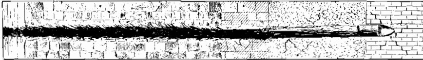
Actual penetration of a trial shot from a 16½-inch, 110-ton gun. The missile passed through 20 inches compound plate, 8 inches wrought iron, 20 feet oak timbers, 5 feet granite, 11 feet concrete, and buried itself 6 feet in a brick wall.
